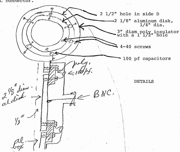
The 80 pf capacitors are aluminum square plates  $13" \times 13"$  held 1/2" from the D surfaces by 4 ceramic staked off insulators. Use 1" long insulators that penetrate clearance holes in the plate as below.
