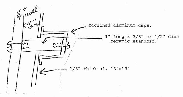
The 1/2 pf coupling capacitors are 1/2 pf ceramic or mica capacitors which connect directly to the dees thru 1/2" holes in the D side.
