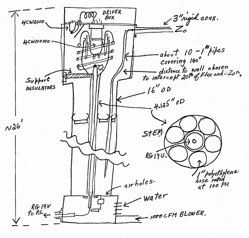
FIG. 4 SKETCH OF TRANSMITTER
