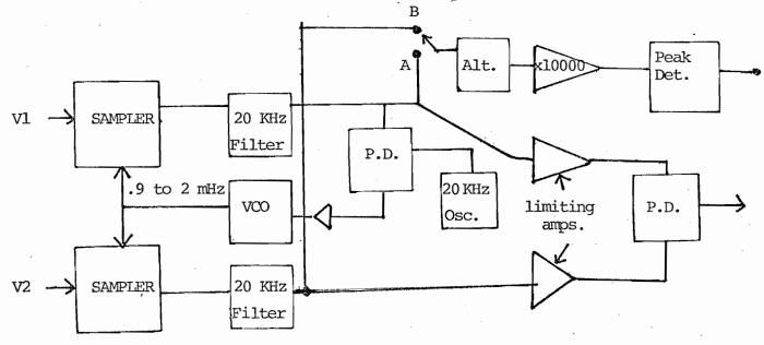
This method is quite satisfactory over a 1000/1 amplitude range, but is  $\underline{slow}$  in that an operator must adjust the gain. It is slow also because the detection is done at 20 KHz and thus the output is limited to a frequency response of about 5 KHz.
