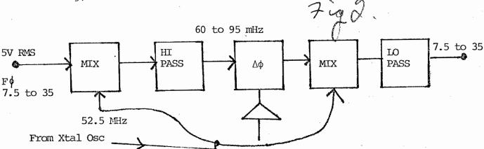
Obviously, this is a perfect way to accomplish phase shifting! The  $\Delta \varphi$  is the same kind of animal as before, but with only a 30%  $\Delta F/F$ . It will work fine. The present phase shifters need only be modified to move the cut-off frequency up to 100 mHz. This means different inductors and varicaps. For the constant K line we are using we must have
