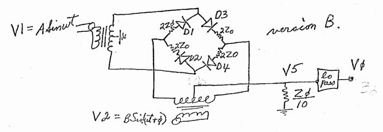
Now if B and  $\phi$  vary, and A is a constant large enough to guarantee turning D1 and D2 or D3 and D4 on hard then both inputs are terminated with a SWVR of less than .05 and we can use it as a mixer, phase detector, or amplitude detector.
