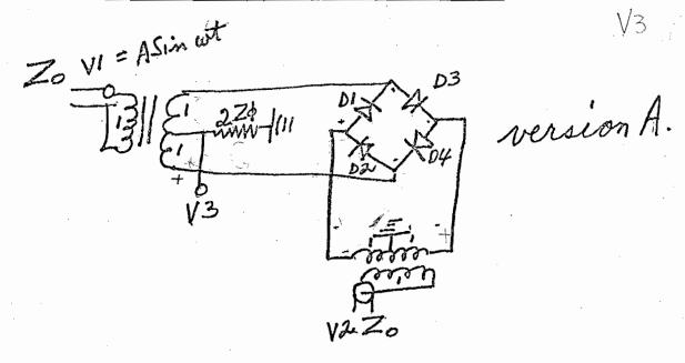
If the diodes are perfect, and VI = V2, then both signals are are terminated and conduction only takes place through diodes D2 and D3, the others being unnecessary and V3 = a full wave rectified signal of amplitude 2A and of average value  $4A/\pi$ . If V2 = 0 then D1 and D2 or D3 and D4 conduct and V1 is short circuited, so for a varying B it is obvious that the above modulator is no good, in fact stupid. So we go to Riedel's balanced, terminated, ring modulator
