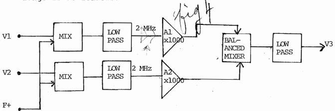
where Al and A2 are limiting amplifiers such that the output square waves are not phase shifted relative to Vl and V2 as a function of the amplitude of Vl and V2. Development work is required to determine if this is possible. Q. Kerns built such amplifiers in 1950 using only vacuum tubes and 1N345 at a frequency of 14 mHz. So I say it is possible to do it now at 2 MHz. It is done with nonlinear feedback. If, as I have heard, one can buy 1GHz opamps, it will be a cinch.
