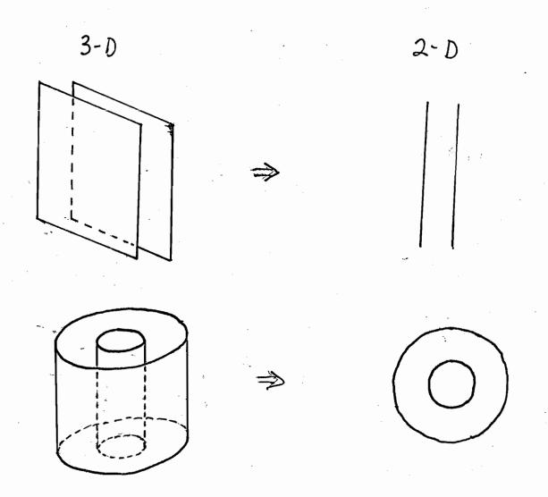
2-DIMENSIONAL REPRESENTATION REQUIRING CYLINDRICAL CORRECTION FACTOR
