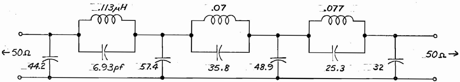
Six filters were built, and frequency data follow. For 70 MHz and below, all filters have phase characteristics within  $10^\circ$ , and below 50 MHz are virtually identical. The pass band amplitude characteristics are flat. At 130 MHz, all filters are at least 60 dB down ( $V_{out} = 10^{-3} V_{in}$ ).
