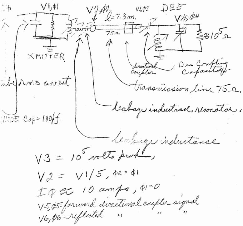
The transmission line when disconnected from the dee and transmitter resonantes in the  $\lambda/2$  mode at 18.3 MHz, corresponding to a length of 8.197 meters or 26.9 ft. There is an anomoly here, as the measured length is more like 7.3 meters corresponding to a mode at 21 MHz. We will resolve this later.
