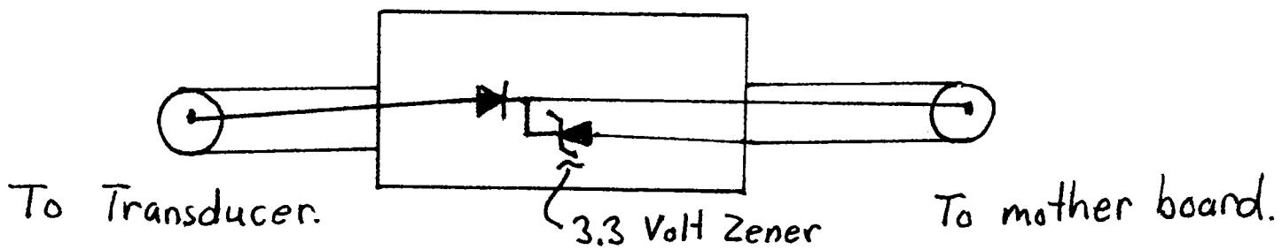
Initially this circuitry was not added to the D.C. over current transducer and we found when the voltage level was increased to approximately 18KV we had additional problems. We determined that allowing any of the trigger signal levels to wildly vary on the mother board did indeed cause cross-talk between signal paths to occur. We eliminated the problem by clamping all signal lines to 3.3 Volts DC maximum. This fix seems to have eliminated the problems.
