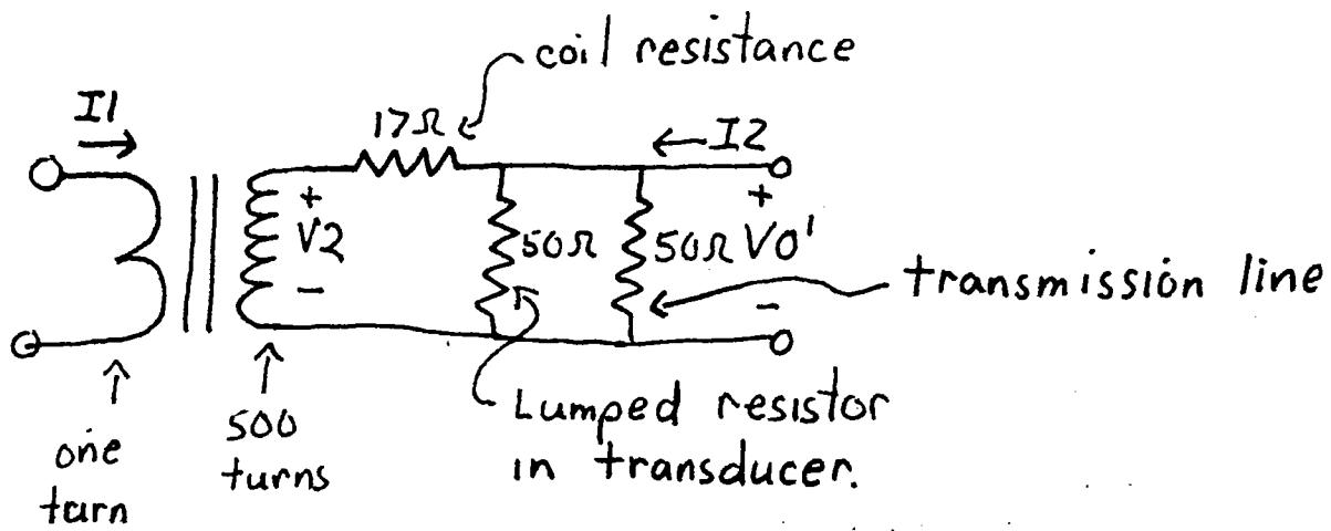
$V_2/V_1 = N_2/N_1 = I_1/I_2$  Coupling coefficient between coils assumed to be 1.
