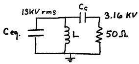
The Q of this circuit is  $\frac{\epsilon}{W}$  where  $\epsilon$  is the circulating energy and w is the delivered power, set at 200 kW.  $\epsilon$ =Vo<sup>2</sup>wCeq. In rf note #80 Ceq could vary from 100pf to 800pf, thus  $\epsilon$  varying from 3 MVA at 28 MHz to 7 MVA at 9 MHz. This corresponds to Q's from 15 to 35.
