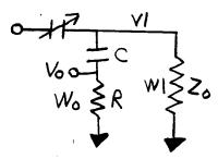
R and C are picked to hold the fundamentals power lost in the resistor to a minimum acceptable level, while simultaneously having a cut-in frequency of just below the transmitter second cavity mode. The frequency where we need to deliver the most power is 27Mhz.
