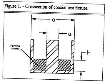
The resistance of the empty fixture is simply due to losses in the coaxial line. When the line is partially filled with a toroid of ferrite material the total resistance is equal to the line section resistance plus the resistance derived from losses inside the ferrite material. The difference then, between the measured resistance of the line with and without the ferrite is simply the losses due to the ferrite material. The difference is written below as
