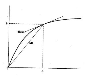
require a much greater variation in H than the parallel case to achieve the same change in  $\mu$ . It is also evident, however, that the perpendicular case will be biased closer to saturation over a given tuning range, and will consequently have lower losses.
