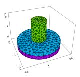
The 2.5D analysis solves the equation  $\nabla \times \nabla \times H_{\phi} - K^2 H_{\phi} = 0$  with the boundary conditions VALUE( $H_{\phi}$ )=0 on the large end and NATURAL( $H_{\phi}$ )=0 on all other surfaces. The natural boundary condition in this case specifies the value of  $n \times \nabla \times H_{\phi}$  that by Maxwell's equations is equivalent to setting the tangential components of E to 0.
